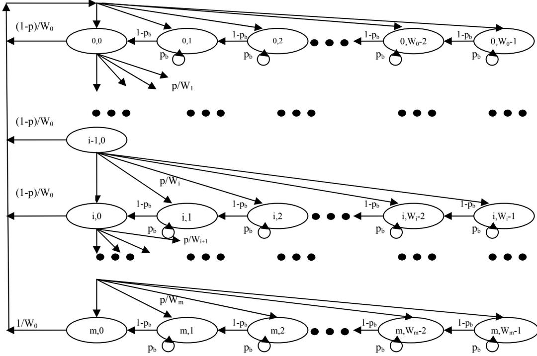
Figure 1. The state transition diagram for the Markov chain model.
