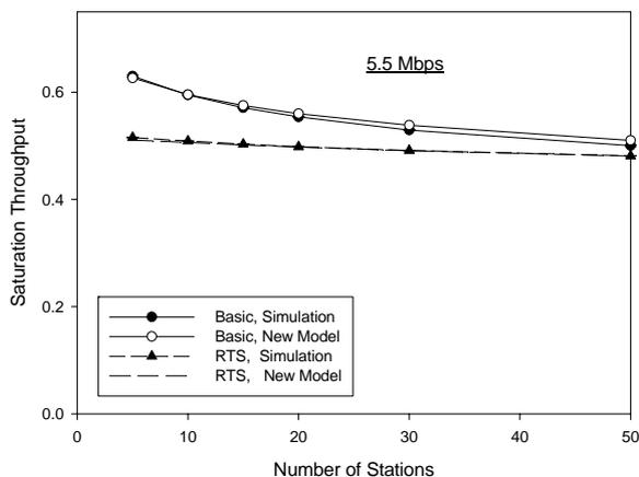
Figure 3. Simulation versus analysis at 5.5 Mbps bit rate for both access mechanisms
