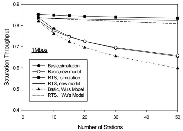
Figure 2. Simulation versus analysis at 1 Mbps bit rate for both access mechanisms
