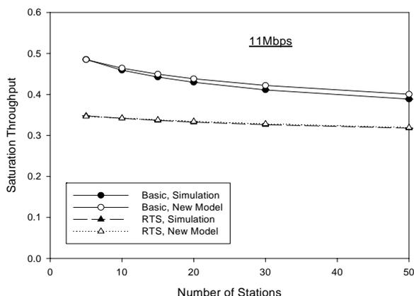
Figure 4. Simulation versus analysis at 11 Mbps bit rate for both access mechanisms
