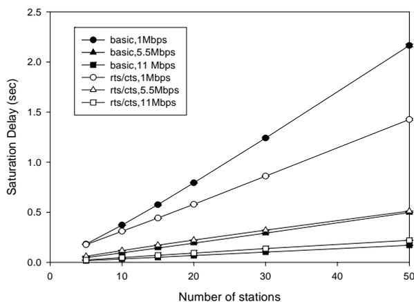
Figure 5. Average packet delay for both access mechanisms.
