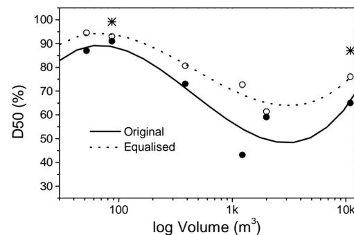
**Figure 7:** Definition (D50) vs Volume of measured acoustic space responses before and after equalization.
