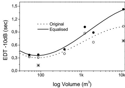
**Figure 8:** Early Decay Time (EDT -10dB) vs Volume of measured acoustic space responses before and after equalization.
