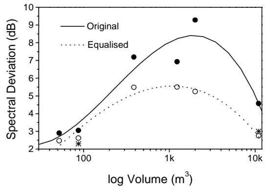
**Figure 10:** Spectral Deviation vs Volume of measured acoustic space responses before and after equalization.
