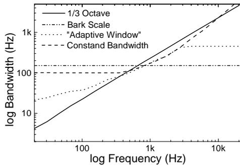
**Figure 1:** Relationship of smoothing bandwidths as function of frequency for various known profiles.
