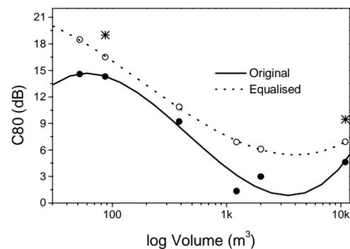
**Figure 6:** Clarity (C80) vs Volume of measured acoustic space responses before and after equalization.
