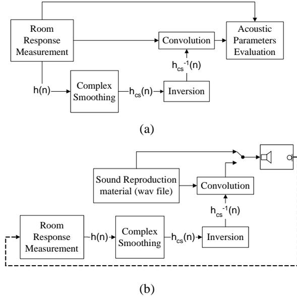
**Figure 5:** Implementation scheme for the proposed equalization method: (a) objective analysis (b) subjective analysis.
