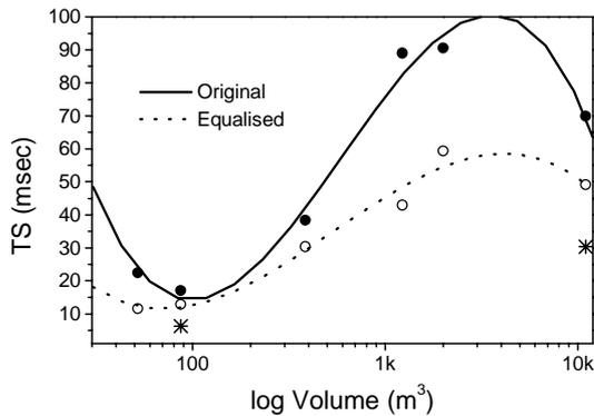
**Figure 9:** Centre time (TS) vs Volume of measured acoustic space responses before and after equalization.
