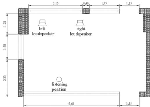
**Figure 4:** Plan view of the laboratory used for subjective tests.
