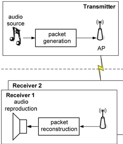
Fig. 1. Configuration of a stereo audio wireless system
