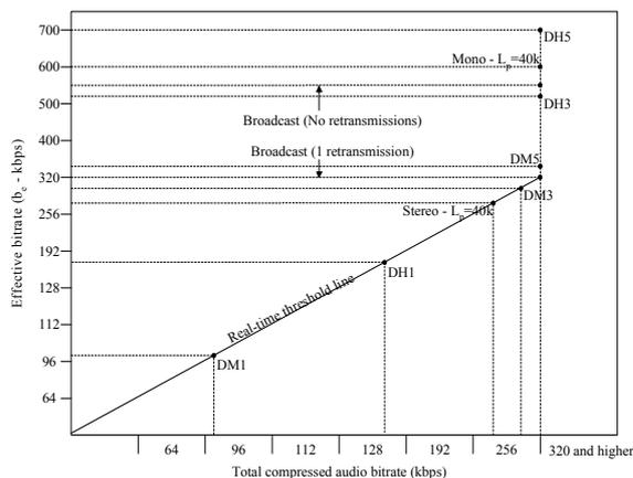
**Fig 4:** Mapping diagram of the audio data bitrate and the maximum allowed compressed audio bitrate for all test cases examined, for 1m distance (from [11])
