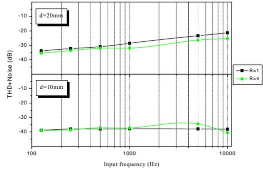
**Fig. 15.** 45<sup>0</sup> measured THD+Noise (dB) for PCM Digital Speaker
