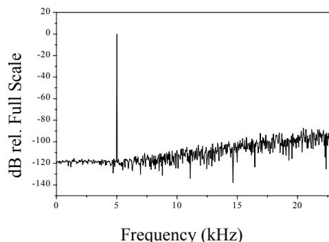
**Fig. 8.** Distortion free PWM conversion using ‘‘Jithering’’ distortion elimination technique
