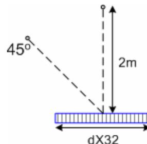
**Fig. 19:** Simulation Positions for the S-D speaker
