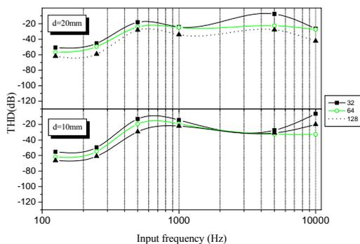
**Fig. 22:** S-D speaker THD vs frequency for different values of R and for the 45° position.
