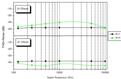
**Fig. 14.** On Axis measured THD+Noise (dB) for PCM Digital Speaker
