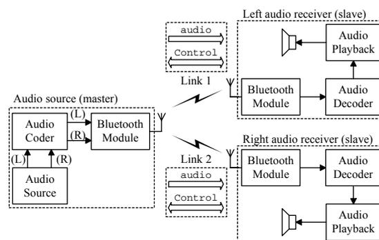
**Fig. 2:** Point-to-multipoint audio and user-controlled information transmission for stereo playback
