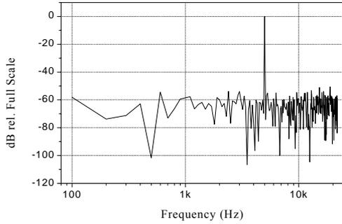
**Fig. 13.** Typical PCM DAE spectrum for 1kHz digital input without oversampling
