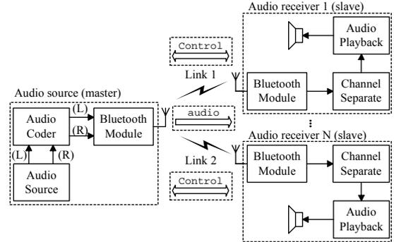
**Fig. 3:** Wireless multichannel transmission using point-to-multipoint connection setup in broadcast mode
