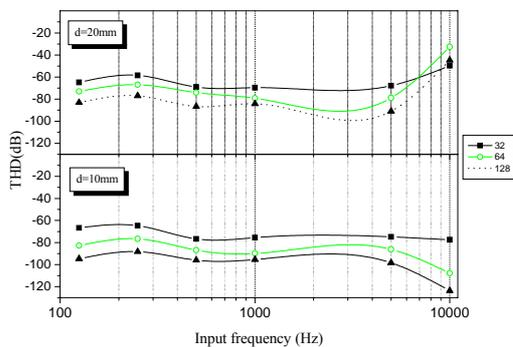
**Fig. 21:** S-D speaker THD vs frequency for different values of R and for the on axis position.
