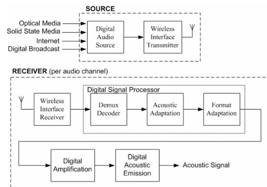
**Fig 1:** Overview of a possible form for the all-digital audio/acoustic chain
