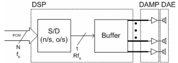
**Fig. 11:** Sigma - Delta Digital Speaker
