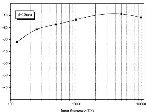
**Fig. 17:** PWM speaker THD vs frequency on axis. The simulation was performed for a distance of 5m and for  $d=10\text{mm}$
