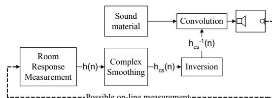
**Fig. 6:** Implementation scheme for the proposed audio/acoustic equalization method.
