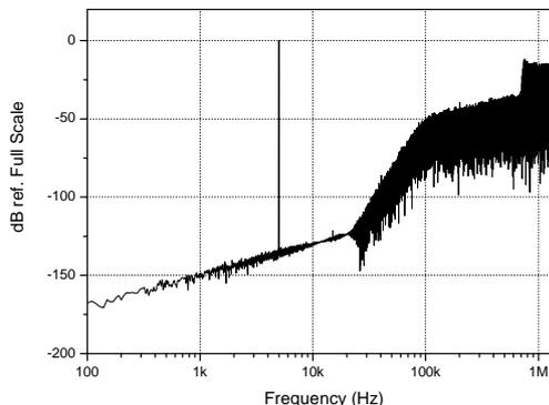
**Fig. 18:** Typical S-D bitstream spectrum
