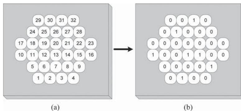
Fig. 3. Typical two-dimensional circular 32-element arrangement and sigma–delta activation pattern. (a) 32-element LA indexing. (b) 32-bit sigma–delta frame activation pattern.
