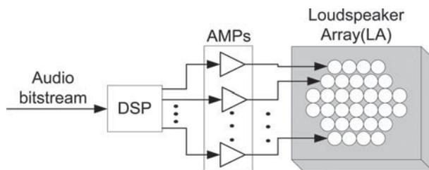
Fig. 1. Typical structure of a DLA system.
