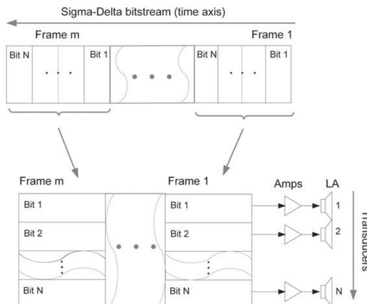
Fig. 2. Typical SDM stream assignment on DLA.
