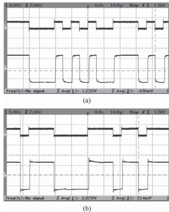
Fig. 6. Input stream and digitally amplified output voltage. (a) Resistive load. (b) Loudspeaker load.
