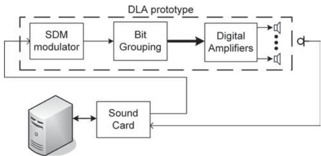
Fig. 9. Diagram of sigma-delta DLA measurement setup.
