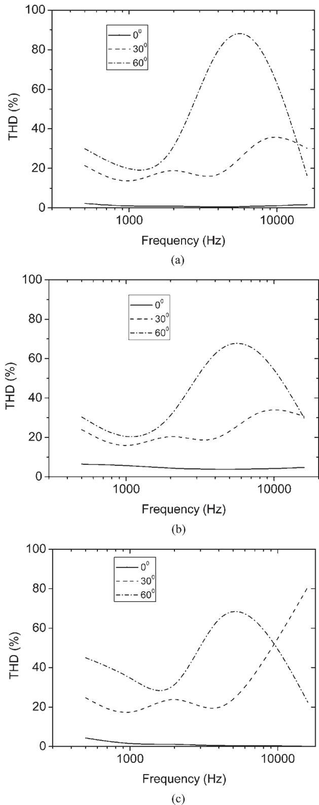
Fig. 11. THD versus frequency for angles of observation  $\phi = 0^\circ$ ,  $30^\circ$ , and  $60^\circ$ . (a) Simulated DLA output for sigma-delta input. (b) Measured DLA prototype output for sigma-delta input. (c) Simulated DLA output for 5-bit PCM input (bit-grouped assignment [16]).
