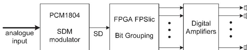
Fig. 4. Architecture of sigma–delta DLA prototype.
