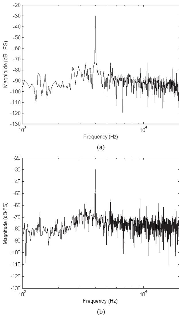
Fig. 10. Sigma-delta pressure spectrum for  $f_{in} = 4$  kHz,  $r = 2$  m audio band. (a) DLA prototype on-axis measurement  $\phi = 0^\circ$ . (b) Off-axis DLA prototype measurement,  $\phi = 30^\circ$ .
