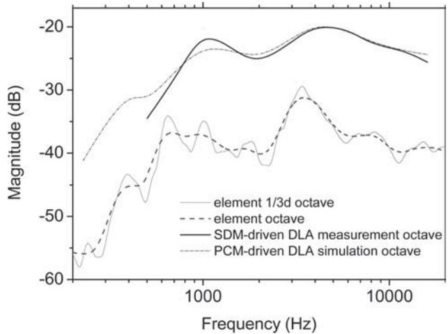
Fig. 8. On-axis frequency responses for one loudspeaker driven by analog excitation (one-third-octave and octave smoothing) and DLA output driven by SDM and PCM streams (octave smoothed). Top curves are shifted vertically for clarity.
