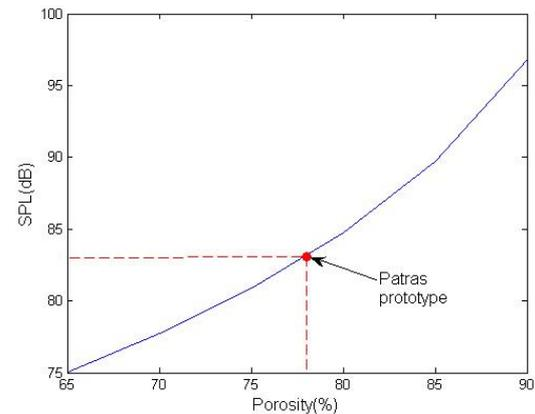
Figure 6 Estimated SPL produced at a distance of 1 m by the thermoacoustic device versus porosity fed with input signal power density of 1 (W·cm<sup>-2</sup>).
