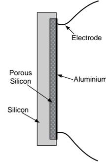
Figure 1 The layers of the solid state thermoacoustic loudspeaker prototype
