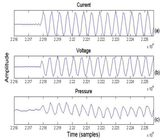
Figure 8 Time response for an 8 (kHz) input signal, measured at a 44100 (Hz) sampling rate. (a) Input current, (b) voltage fed to the device and (c) generated acoustic pressure
