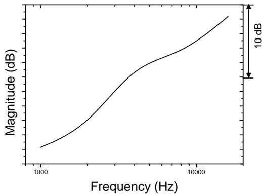
Figure 10 Measured frequency response of the thermoacoustic device
