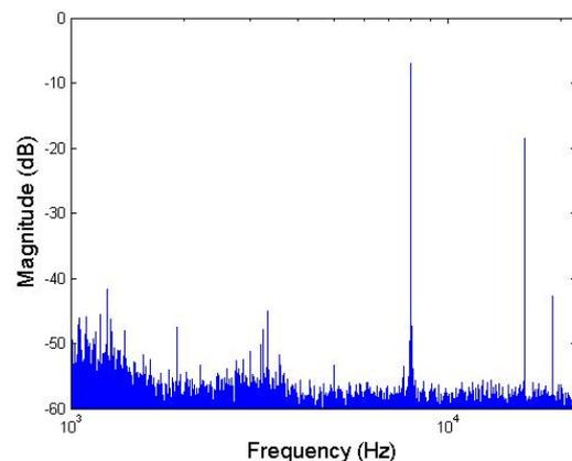
Figure 9 Pressure spectrum for an 8 (kHz) signal reproduced by the thermoacoustic device
