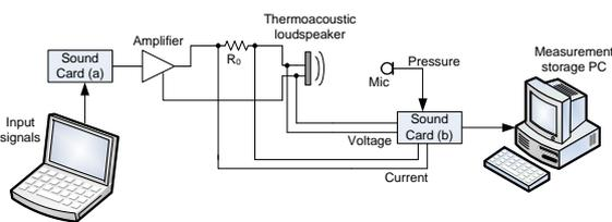
Figure 7 Prototype measurement setup
