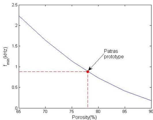
Figure 4 Minimum frequency reproduced as a function of porous silicon layer porosity for a thickness of 10.7 μm
