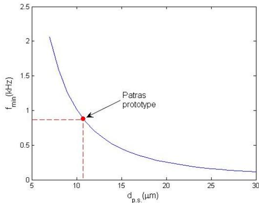
Figure 3 Minimum frequency reproduced by a thermoacoustic loudspeaker as a function of porous silicon layer thickness
