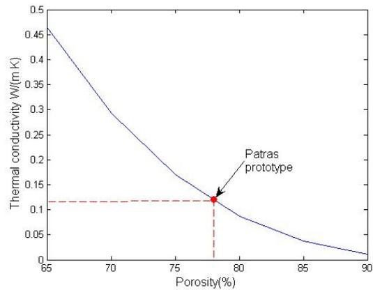
Figure 5 Thermal conductivity of the porous silicon layer versus its porosity
