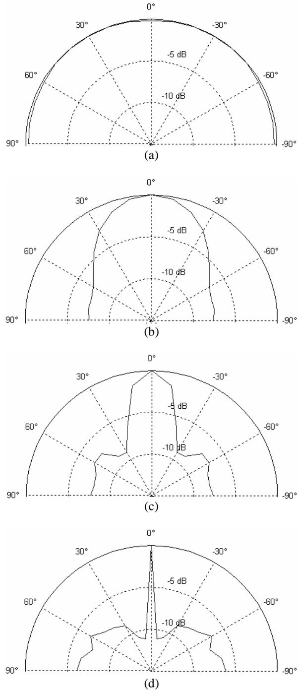
**Figure 12** Linear DLA Directivity (a)  $f_{in}= 250Hz$  (b)  $f_{in}= 1KHz$ , (c)  $f_{in}= 2KHz$ , (d)  $f_{in}= 10KHz$ ,  $l=2m$
