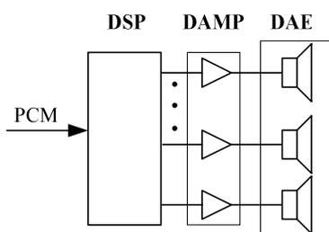
**Figure 1** Digital Loudspeaker Array structure
