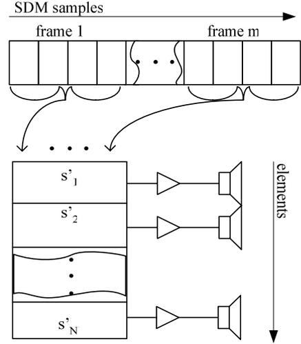
Figure 2 Bitstream grouping and emission
