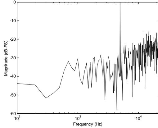
**Figure 10** Pressure spectrum, Linear DLA
